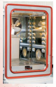
An essential element of the climatic system of the chambers is the humidification bath. This technology guarantees economical consumption of water, quick reaction times and long-term tests.
